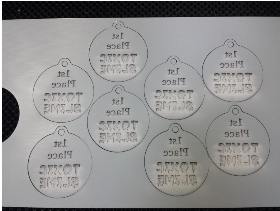
Flipped text engraved from the back
