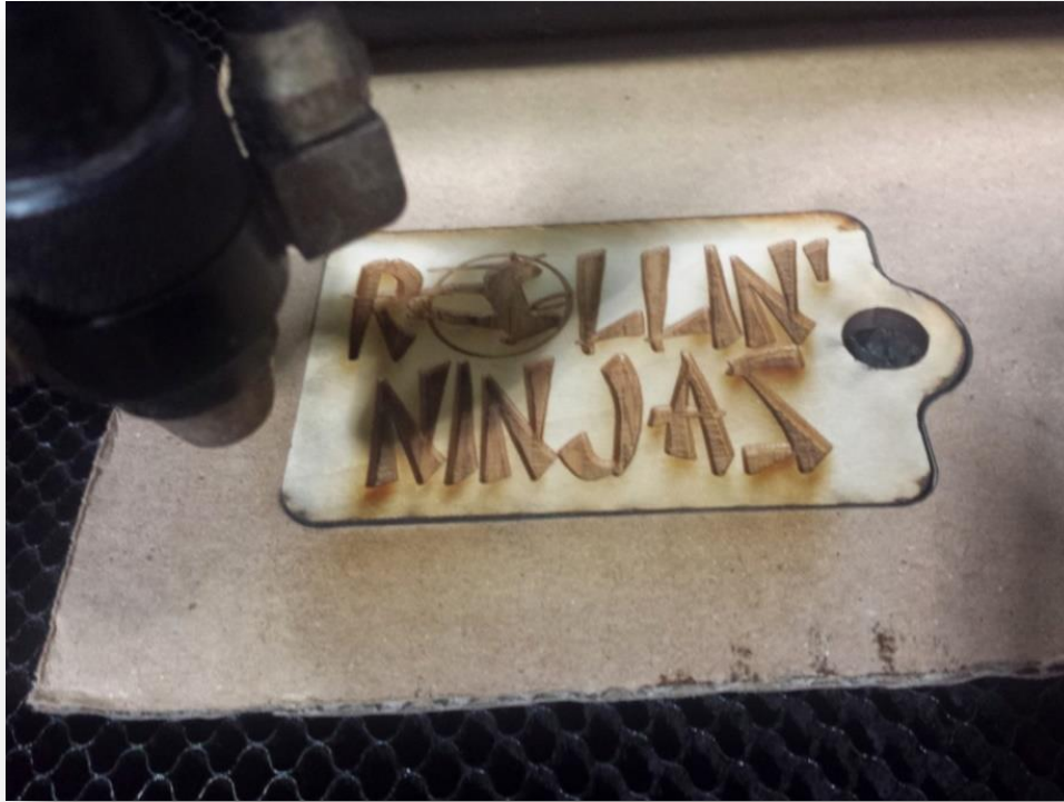
Engraving the Back Side in the Jig
