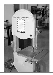
14" Bandsaw: Used for cutting curves and shapes in lumber. The foot needs to be within 1/4" of the material being cut. Never force your material into the blade, let the machine do the work (forcing material results in weakening and eventually breaking of the blade). Keep your fingers out of the path of the blade when cutting!
