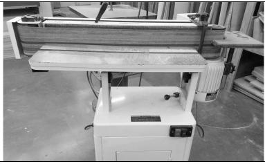
Edge Sander: Used to sand edges and shapes. This machine is not intended, nor is it capable of producing straight, even edges. Always keep your material flat on the table. Always sand against the rotation of the belt (from right to left). Do not force material against this machine as it will ruin the belt!!! This machine will remove a lot of material very quickly, so be aware. Lumber only is allowed on this machine! No sheet goods! Watch your fingers!
