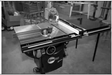
Dado Saw: Used to mill dadoes and rabbets in material. Stock must be at least 12" long and you need to use a push stick or pad when cutting stock. The blade cannot be seen when milling dadoes and rabbets so use extreme caution!!! The long edge of the board must be against the fence. Slow and consistent feed rates are required! You must always use two push pads when using the dado saw!
