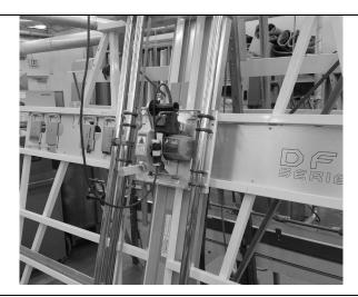
**Panel Saw:** Used for cutting larger sheet goods to *rough* size. Do not expect this machine to accurately cut to finished dimensions! Allow the saw to do the work and do not force the saw through the material. Always clamp smaller pieces to the machine prior to cutting. This machine is intended to mill larger, difficult to handle material down to a more manageable size.
