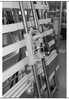
**Panel Router:** Used for routing dadoes and rabbets in larger pieces of material. Sheet goods are clamped in place and the router is moved vertically to create the dado or rabbet. Take care to adjust the location of cut and the bit depth accurately. A minimum of 2 clamps are required to hold your material securely when cutting. Do not force the router through the lumber; let the bit do the work.
