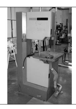
Resaw Bandsaw: Generally used for resawing solid lumber to thickness and cutting of large / thick stock. The foot needs to be set within 1/4" from the stock while cutting. No adjustments are to be made to the blade guides by students. Never force material into the blade, let the machine do the work (forcing material results in weakening and eventually breaking of the blade). Keep your fingers out of the path of the blade when cutting!
