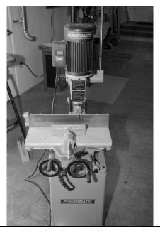
**Mortise Machine:** This machine is able to drill square holes (a mortise) used in mortise and tenon joinery (square peg in a square hole). Bits are available in various sizes to match the particular need. Do not force the cutting action and if the bit begins to heat up stop to allow it to cool down before proceeding.
