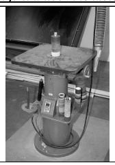
**Spindle Sander:** Used for sanding shapes and irregular pieces. Always keep your material flat on the table. Watch your fingers! *Spindles are to be changed by instructor only!!! Do not force you material against the spindle! Move your material against the rotation of the spindle.*
